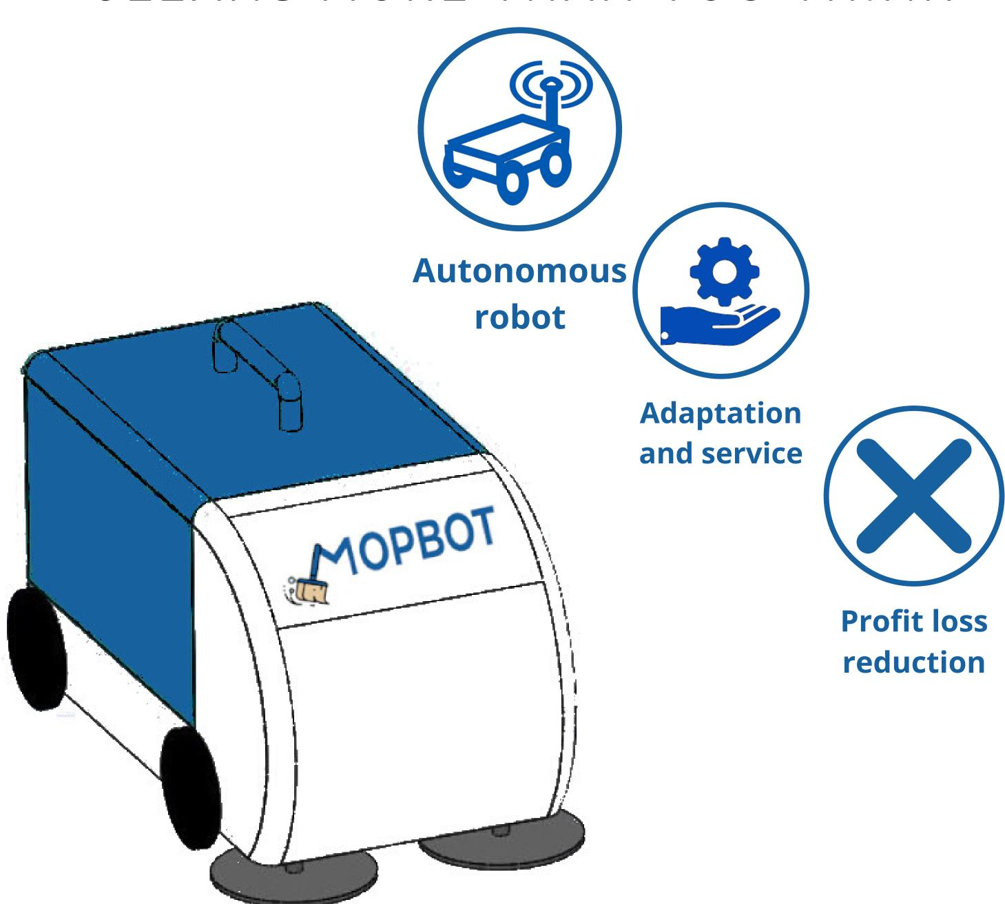
Mopbot is a cleaning robot for the floor area of industrial facilities. Eliminate small rubbish and dust that is left behind after a day of trading using two vertical brushes on the front and a vacuum system.
